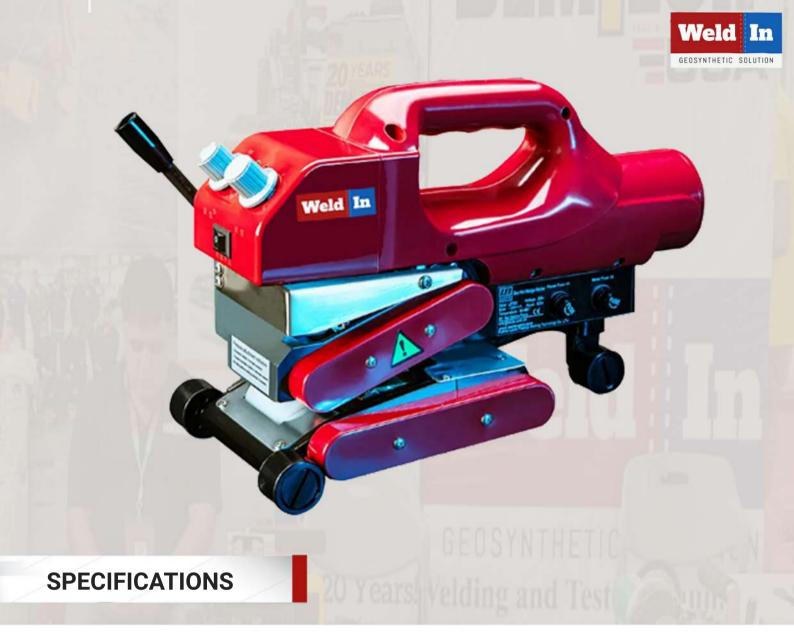
Model Rated Voltage Rated Power Frequency Heating Temperature Welding Speed Material Thickness Welded Seam Width 1 Weld Strength Overlap Width Digital Display Body weight Warranty Certification WIN 800 230V/120V 800W/1100W 50/60HZ 50~450 0.5-5m/min 0.2mm-1.5mm(single layer) 2.5mm\*2,Interior Cavity 12mm  $\geq$  85%material 10cm No 5kg 1 year CE
