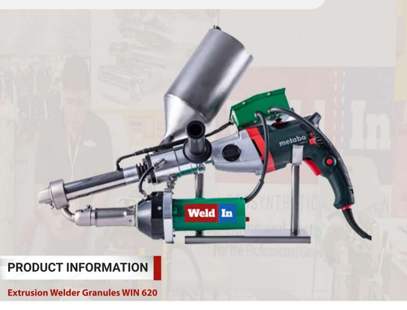
This plastic extrusion welder is the first plastic granules extrusion welder in China that has functions of double independent heating systems, digital display controller, 360-degree rotating welding head, motor cold start protection, which is applicable to welding PE, PP and other hot melt materials
